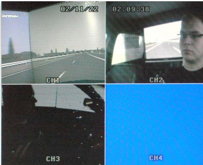
Fig. 8: View on the driver during experiment, recorded using 4 cameras (the blue one is normally used for visual record of outputs from psycho-physiological measures)
