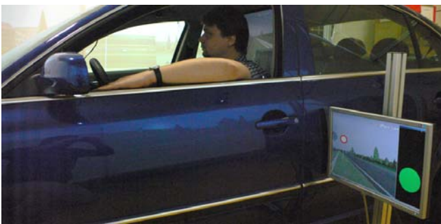
Fig. 5: Implementation of the left rear mirror – it is possible to see the projected picture with semaphore (see the chapter concerning the experiments)
