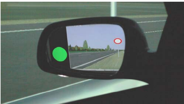
Fig. 6: Driver's view into the left mirror – including the semaphore (see the chapter concerning the experiments)
