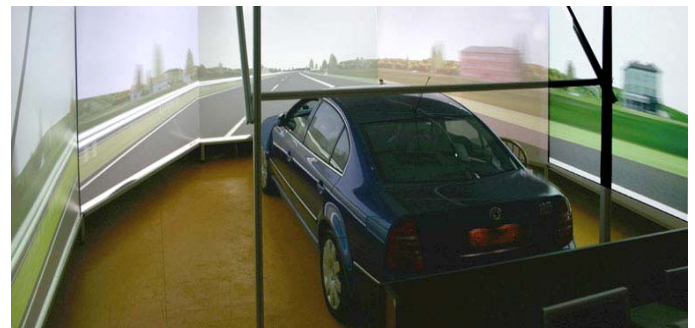
Fig. 2: Our driving simulators with 5 projection screens covering 210° of driver's view
