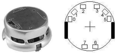
Figure 1: The Khepera robot. A schema of sensors and motors within the robot body.
