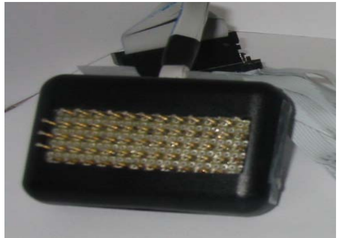
Fig. 3: 2D matrix (13 rows and 5 columns) of surface electrodes used for sEMG acquisition.
