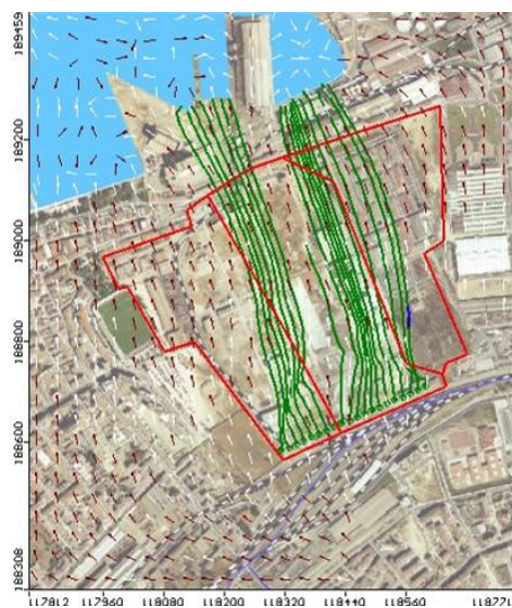
Fig.13 – Dynamics of local groundwater flow and path of a contaminated plume (in [2])
