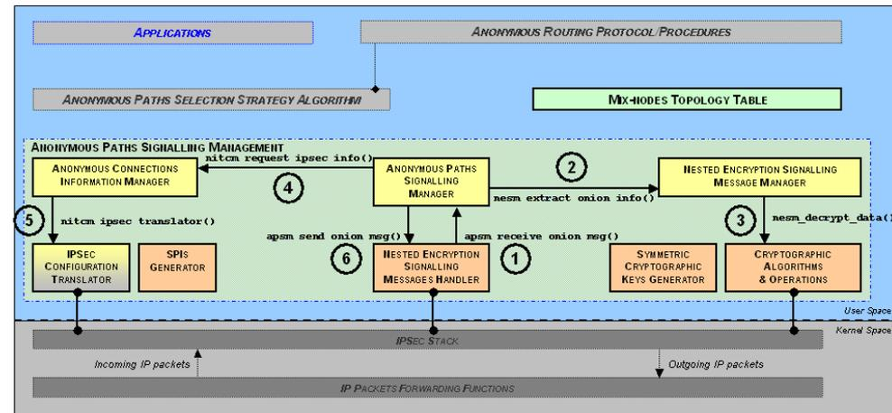
Figure 5. Treatment of an anonymous path signalling message by the APM software components.
