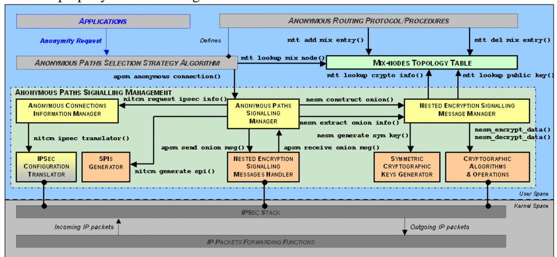
Figure 3. Software architecture of the APM module.
