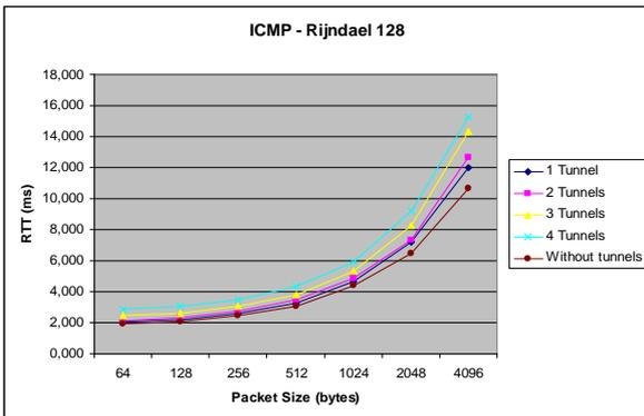
Figure 8. RTT vs. Packet Size using Rijndael 128.
