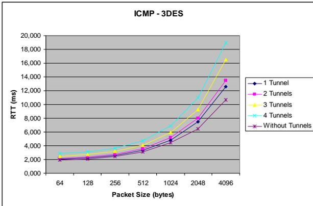
Figure 7. RTT vs. Packet Size using 3DES
