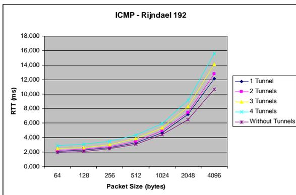
Figure 9. RTT vs. Packet Size using Rijndael 192.
