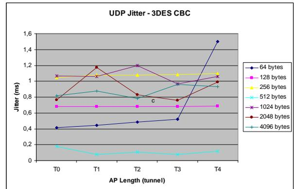
Figure 11. Jitter vs. Anonymous Path Length using 3DES.
