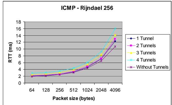
Figure 10: RTT vs. Packet Size using Rijndael 256
