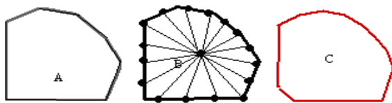
Fig.2 Radial casting of irregular shape
