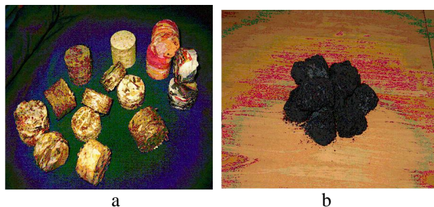
Fig.1 Different types of waste raw briquettes (sawdust, cotton, paper, cereals) and soybean hulls char.
