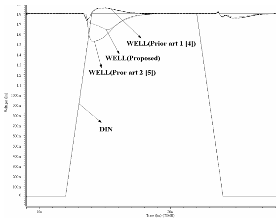
Fig. 10 The comparison of the WELL voltage among the proposed circuit, prior art circuit [4] and prior art circuit [5] as an output buffer at 50MHz
