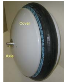
Fig. 1: Gyrobot in its vertical position
