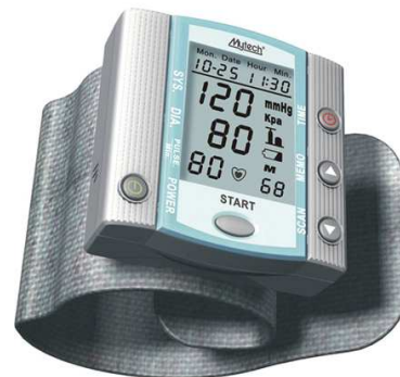
Fig. 9. The wireless sphygmomanometer and pulsimeter prototype
