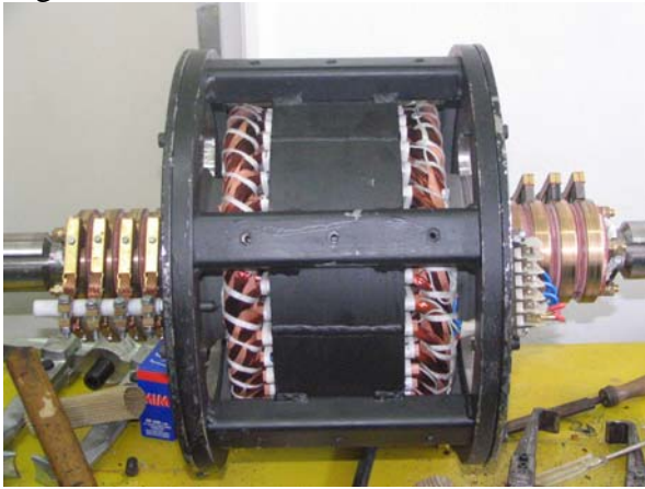
Fig.1 Inverted rotor induction motor construction
