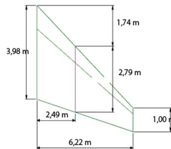
Fig.3 Horizontal Tail Geometry
