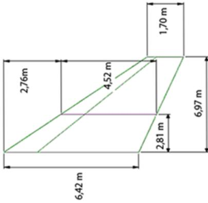
Fig.4 Vertical Tail Geometry
