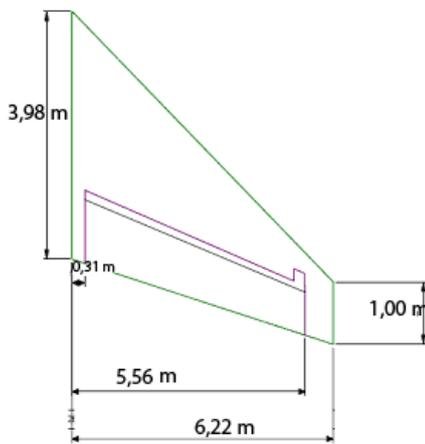
Fig.6 Elevator Geometry
