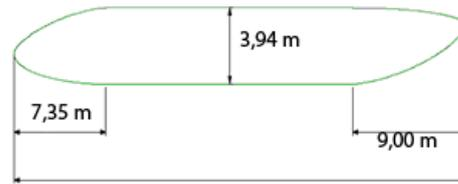
Fig.1 Fuselage Geometry
