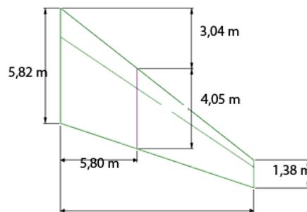
Fig.2 Wing Geometry
