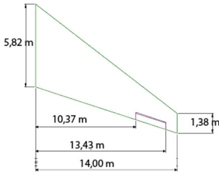
Fig.5 Aileron Geometry
