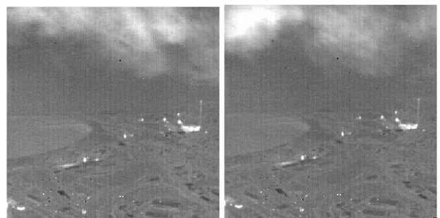
Fig.1 – Two successive frames of infrared imagery showing large changes in image noise from aircraft exhaust plume at the top of each image.
