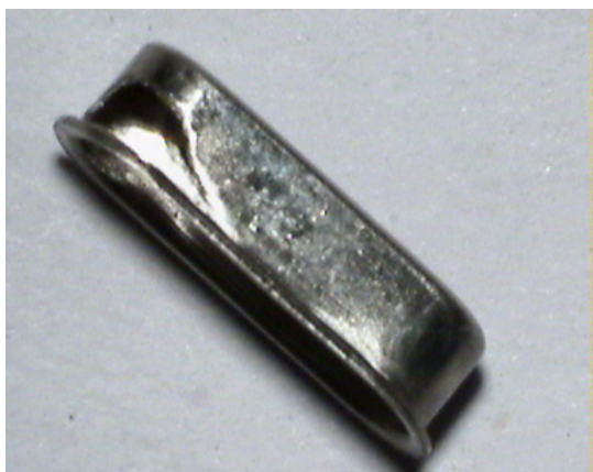
(a) The broken cover
