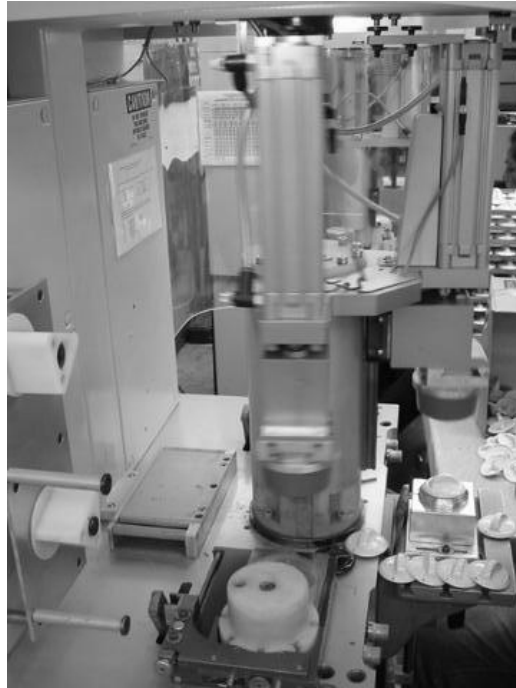
Figure 1: The stamping machine with the kitchen knobs on the right hand side.
