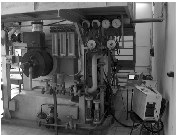
Fig. 6 Gaseous and liquid fuels furnace view; Thermal and nuclear equipment chair laboratory
