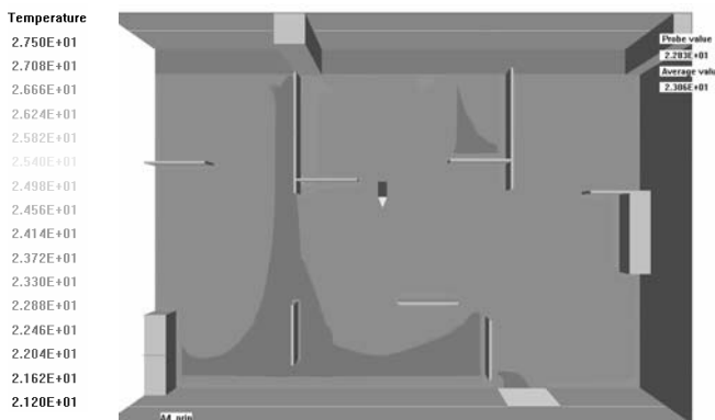
Figure 5. Plan view of temperature at z=1.5m (Basic)
