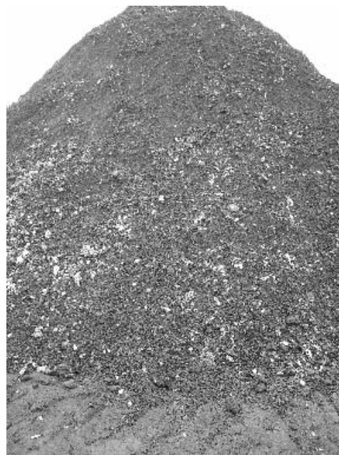
Fig.1 View of the mix of the formed fuel and coal in the yard (M-I mix).
