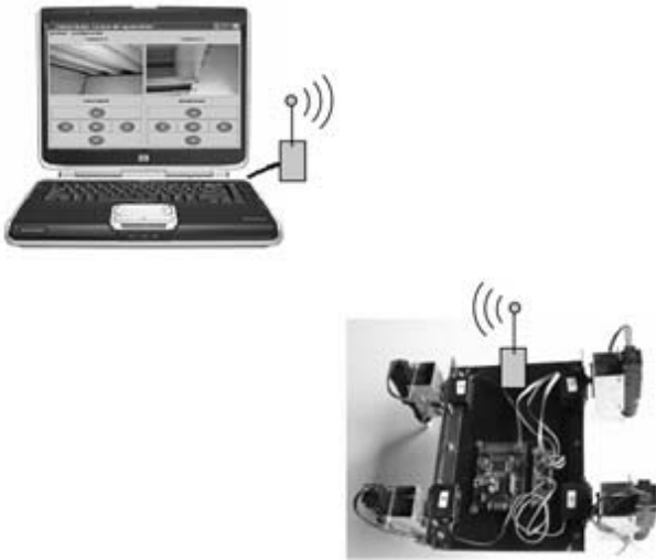
Fig. 9.- The graphical user interface to control the robot performance and display data and visual information.
