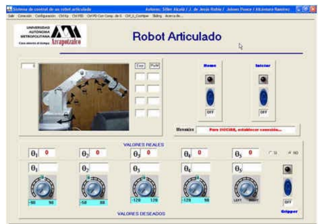
Figure 8 The graphical user interface developed in Visual Basic 6.0
