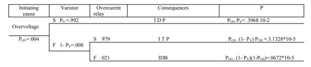
Fig 7 The reduced ETA for initiating over-voltage event
