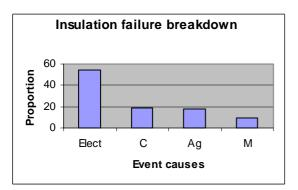
Fig.3 Insulation failure modes distribution
