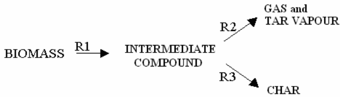
Fig.1 – Model of pyrolysis mechanism with intermediate compound [1]
