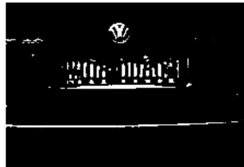
Fig. 3. Resultant binary image after hat transformation, and removing small features from the resultant hat image.
