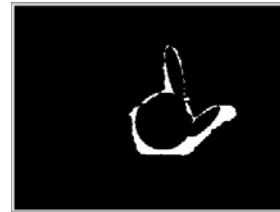
Fig. 8: exor between the projection of the model and the silhouette of the hand
