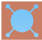
Fig. 8: Bolt hole slots, ending with small circular gaps
