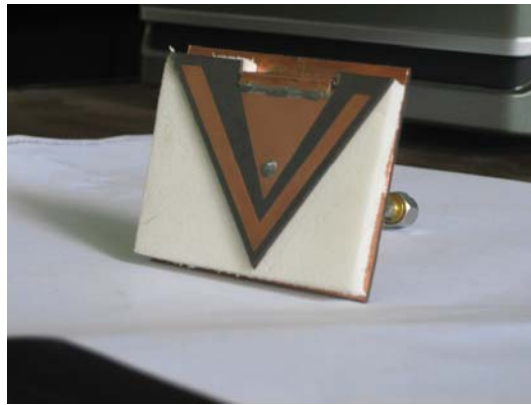
Fig.2: Photo of the fabricated proposed antenna for six multi-band operations
