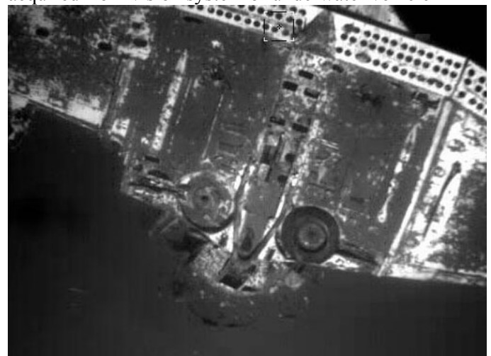
Fig.4. The results of unplait operation applied to the image obtained by vision system of underwater vehicle
