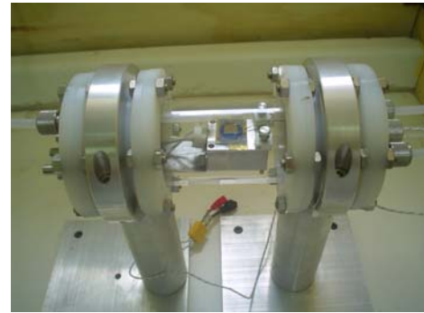
Fig. 2. Hermetic reactor used to sense the response of the organic vapors.
