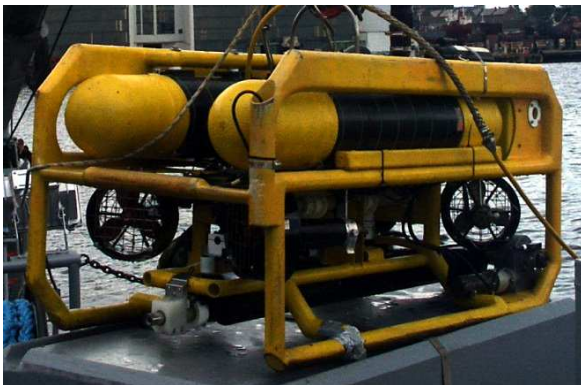
Fig. 5. Object of research - remotely operated, underwater vehicle "Ukwial"
