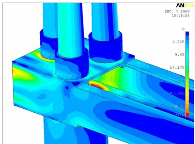
Fig. 5 Von Mises stresses during AF2 seism [MPa] (zone of maximal stresses)
