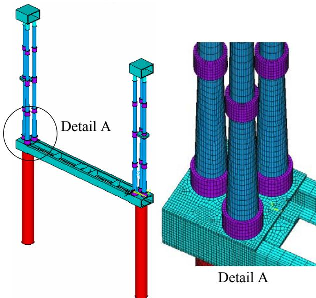
Fig. 2 F.E.M. model of the disconnector
