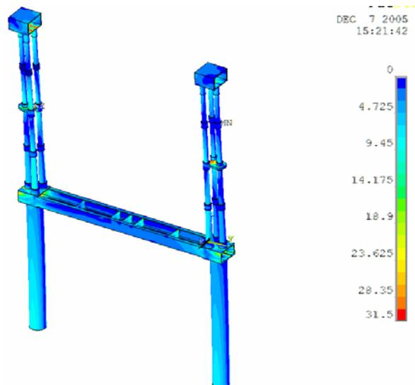
Fig. 4 Von Mises stresses during AF2 seism [MPa]
