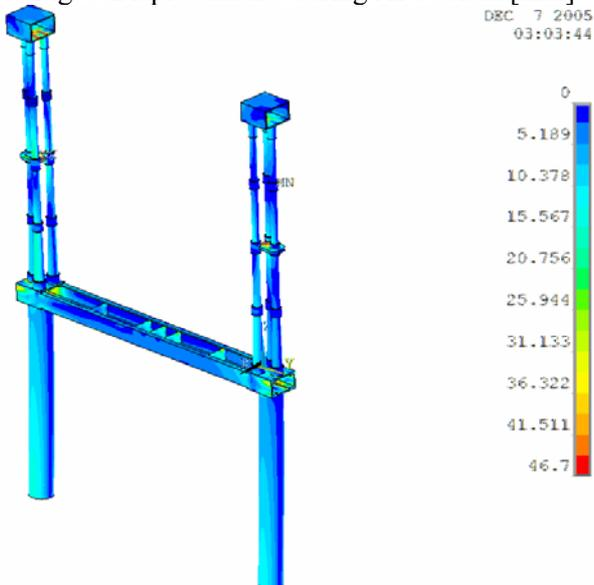
Fig. 7 Von Mises stresses during AF3 seism [MPa]
