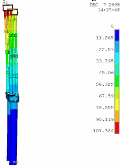
Fig. 6 Displacements during AF3 seism [mm]
