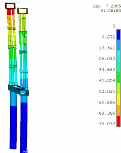
Fig. 3 Displacements during AF2 seism [mm]
