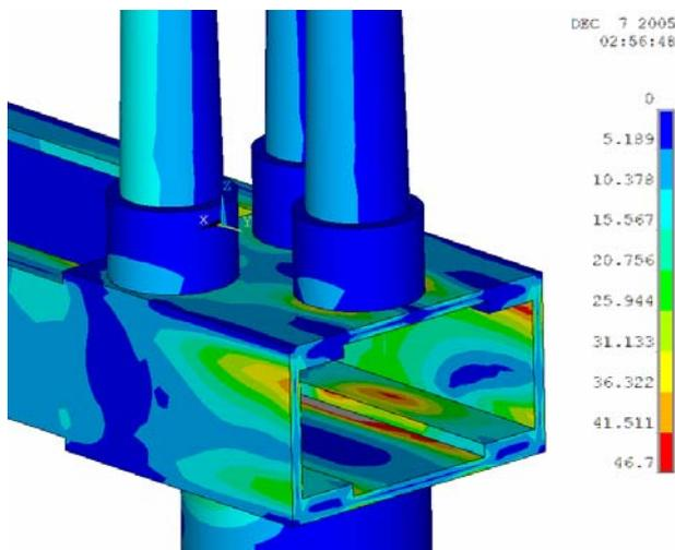
Fig. 8 Von Mises stresses during AF3 seism [MPa] (zone of maximal stresses)
