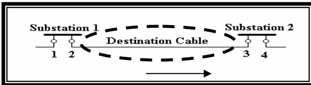
Fig. 4: Case 1: The cable is between two normal substations.
