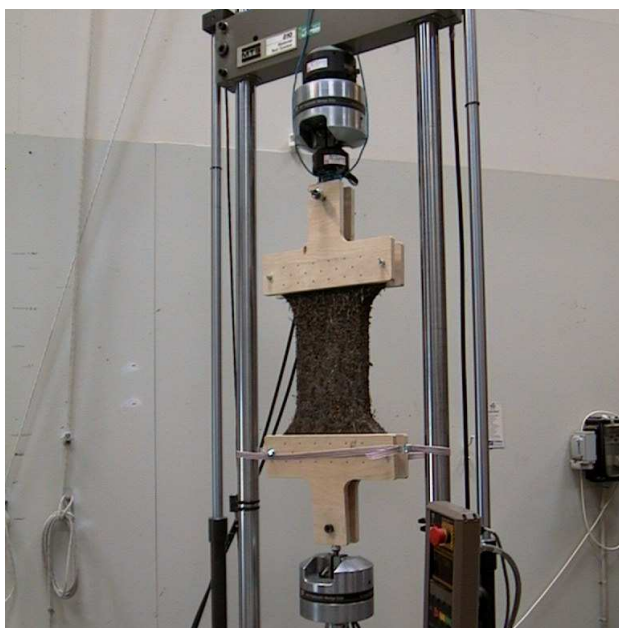
Fig. 2. The test specimen is fastened in a testing machine and pulled apart at a constant crosshead speed of 10 mm/min until failure occurs.
