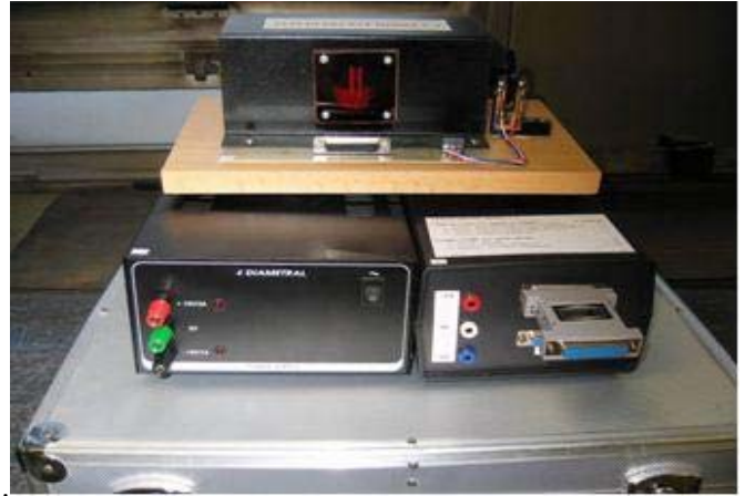
Figure 3 Photo of the final version of an experimental HAA model in mobile form with portable case (5 prototypes were produced)
