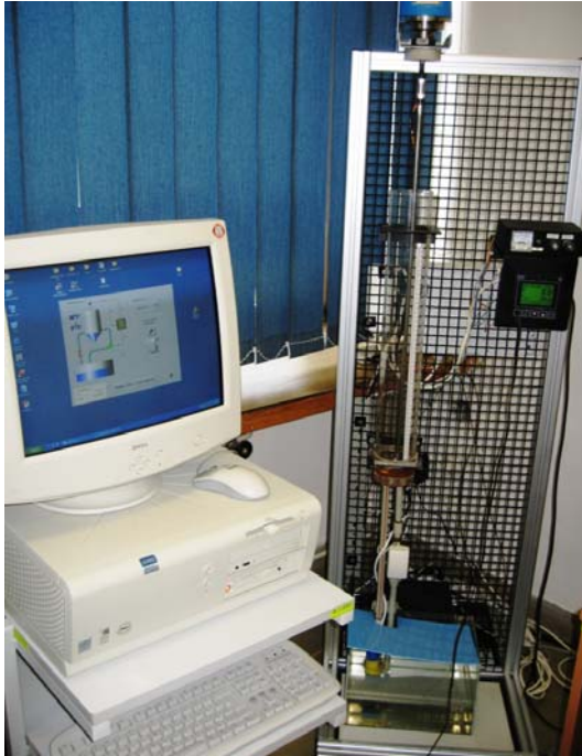
Fig. 8 Model of level tank control with an industrial controller in connection with a PC
