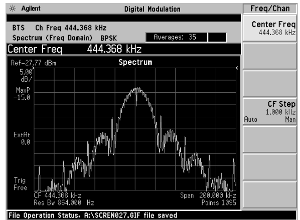
Fig 13 : Spectrum with a simple R,C filter
