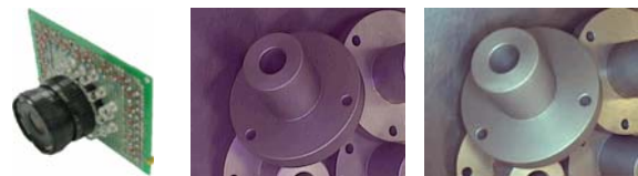
(a) Lighting system (b) Image without (a) (c) Image with (a) Fig. 3 The lighting system and an acquired image compared to the one obtained without the light system
