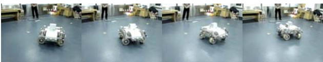
Fig.12 Test of robot rotates around the point where wheel 4 contacts with ground
