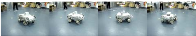
Fig.13 Test of robot rotates around the point which locates within supporting area
