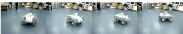
Fig.15 Test of robot rotates around the point locates at the sharp rear exterior supporting area
