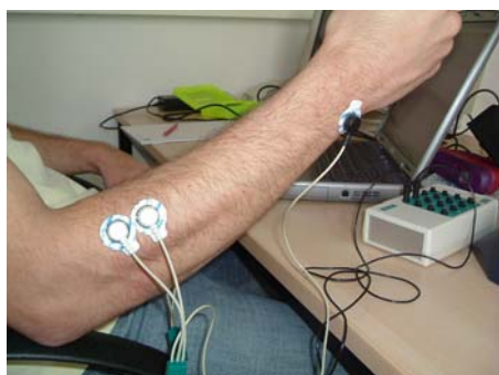
Fig. 1: EMG training and test patterns recorded using two pairs of electrodes in Max Planck Institute laboratory in Magdeburg, Germany.
