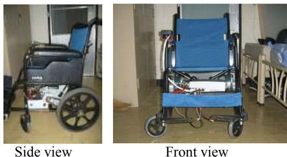
Fig. 1 Speech voice commanded automatic wheel chair.
