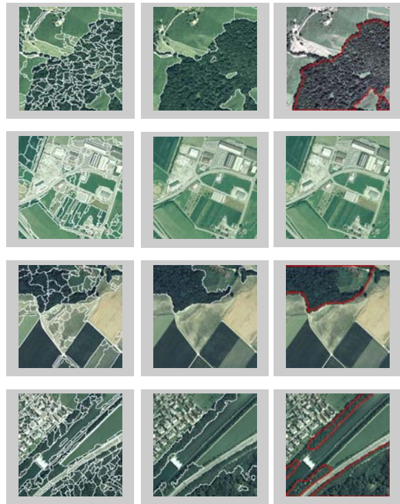
Fig. 9a JSEG segmentation Fig. 9b final forest boundary detection Fig. 9c manual interpretation of forest
