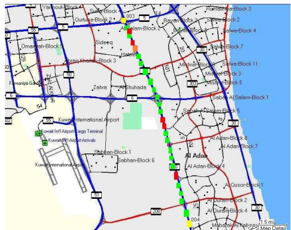
Figure 5. Magnetic radiation level along the King Fahad road from NCC to Qosour for trip 4.
