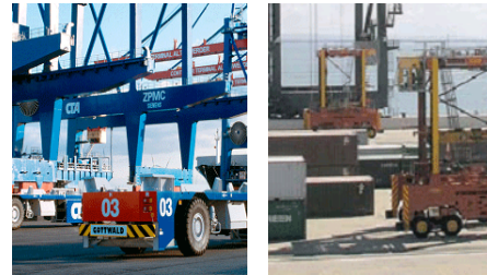
Fig. 1 Automated transportation equipments for ACT-AGV, ASC
