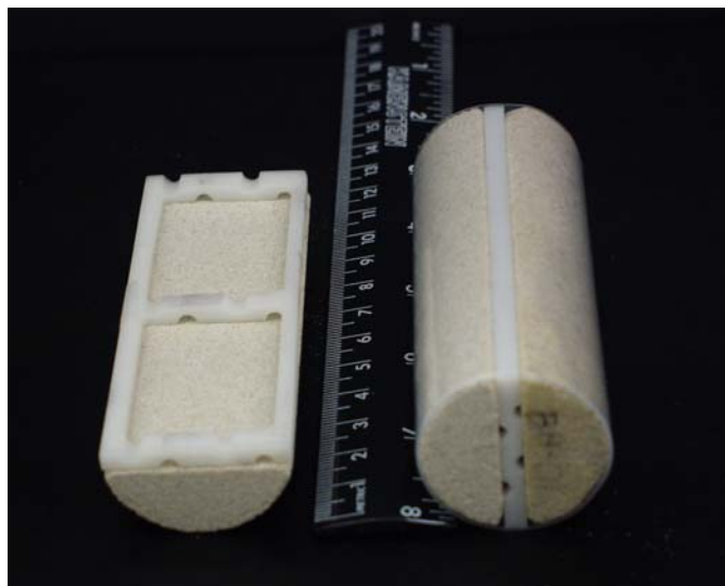
Fig. 2; Picture of fractured core and spacer
