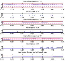
Fig. 2. Room & System States after Coordination. A system consisting of 10,000 cool rooms with large variations in parameters has been set up to test coordination performance and scalability. The cool rooms have the same temperature constraint, but diverse power capacities and time constants, random starting internal temperatures, and random initial switching states for the cooling plan.
