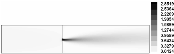
Fig.6 Velocity Contours (m/s) at symmetry plane
