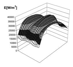
Fig.3. Irradiance distribution  $E [W/m^2]$  on a furnace wall for heat coil (H=60mm and r=8mm)
