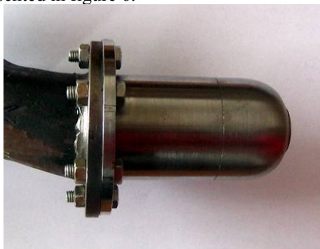
Fig.6 The new injector for Pelton turbine
