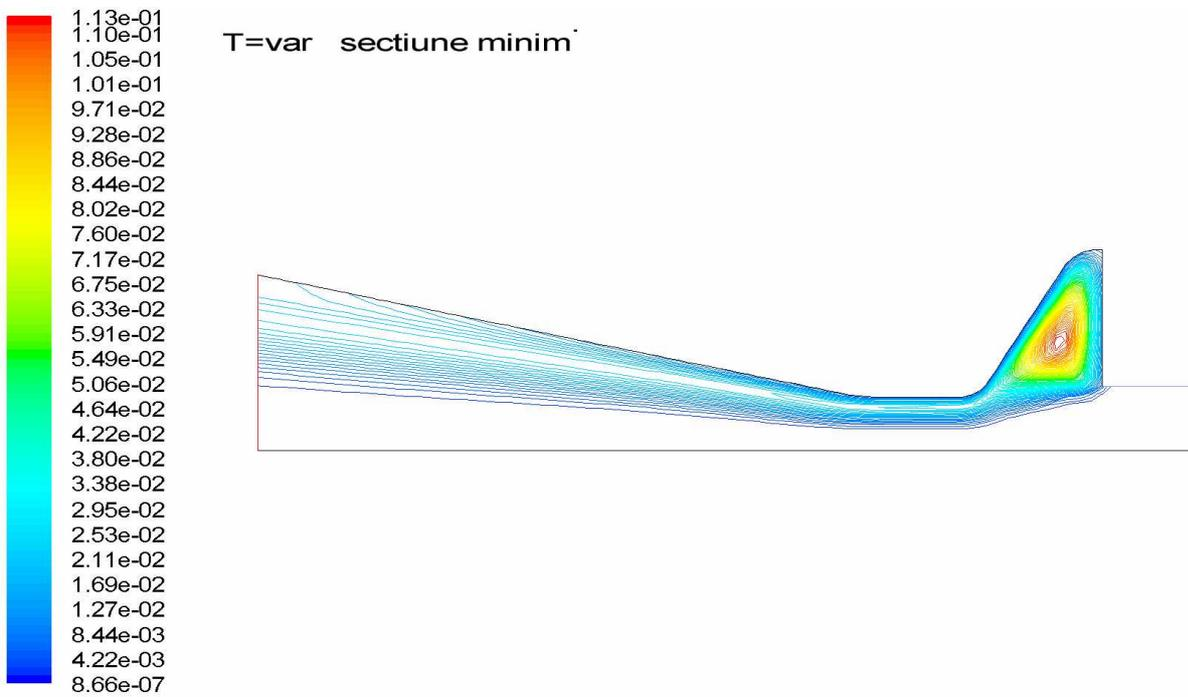
Contours of Modified Turbulent Viscosity (m2/s) Feb 26, 2006
