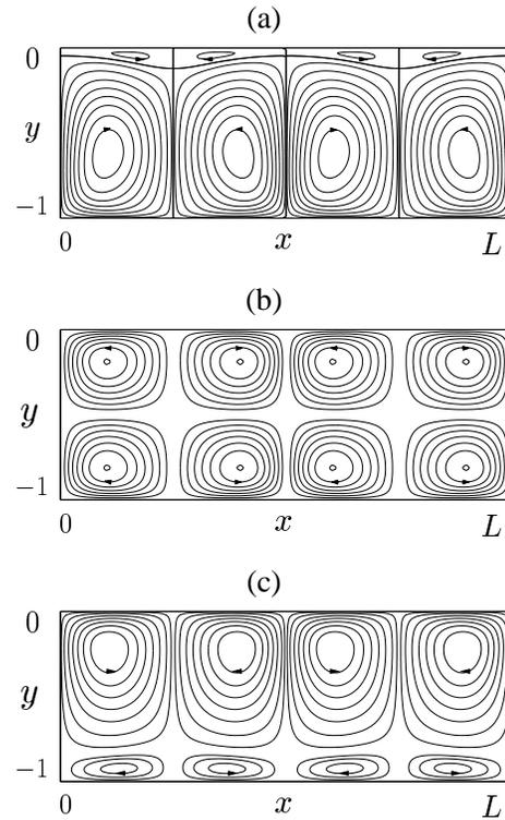
Figure 3: Mean flow streamlines of (14) for the basic standing waves solutions for different values of the film parameter  $\Gamma$ , for  $k = 2.37$ ,  $L = 2.65$  ( $m = 1$ ), and  $(\tilde{Re}, \Gamma)$ : (a) (200, 0.1), (b) (160, 0.5), (c) (60, 0.9).
