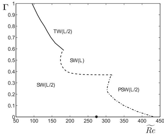
Figure 4: The primary instability of the basic SW for different film parameter values for  $k = 2.37$ ,  $L = 2.65m$  (checked for  $m = 1, 2, \dots, 10$ ). The bifurcation is either a Hopf bifurcation ( $-\cdot-\cdot-$ ) if  $0 < \Gamma < 0.371$ , a  $(L/2)$ -symmetry breaking bifurcation ( $---$ ) if  $0.371 < \Gamma < 0.588$ , or a parity breaking bifurcation ( $---$ ) if  $0.588 < \Gamma < 1$ .
