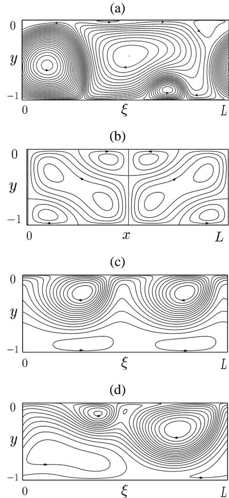
Figure 5: The streamlines for some representative steady (b) and steadily travelling ((a),(c) and(d)) attractors of (14), for  $k = 2.37$ ,  $L = 2.65$  ( $m = 1$ ) and the following values of  $(\widetilde{Re}, \Gamma)$ : (a) (2000, 0.2), (b) (200, 0.5), (c)(200, 0.9), and (d) (600, 0.9). The streamlines of (a), (c) and (d) correspond to moving axes  $\xi = x - \psi'\tau$ , with the constant drift velocity  $\psi' = -0.1382, -0.072, \text{ and } -0.097$ , respectively.
