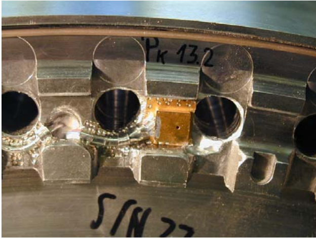
Fig. 5: Pressure Sensor At Receiver Inlet
